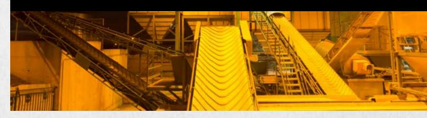
Incline belting is used in high-incline environments, utilizing cover textures and vulcanized profiles to keep transported materials secure while in motion. With an array of different compounds available for fabrication, incline belts can be implemented with virtually any application.
