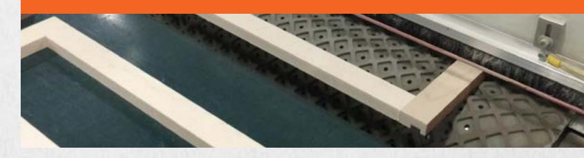
We offer the best belting for surface finishing, serving wood and metal finishing industries. Our belts are designed specifically to meet OEM requirements and we offer the clear top choice belt of Cabinet Sander OEM's worldwide. Our carcass constructions utilize a variety of cross rigid properties to resist edge curl and provide a flat, stable carrying surface for wood panels and metal parts.
