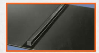
Magnetic separator belts revolve around a magnet suspended over a conveyor. These magnets attract unwanted scrap metal from the material being conveyed and pull the metal up against the belt. With the help of cleats, the unwanted metal is transported out of the magnetic field and discharged into a collection area. These belts are available in rubber, urethane and PVC.
