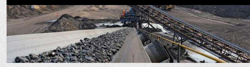
More than 50 separate types of heavy-duty black rubber belt specifications are available for cut flat belt or custom-fabricated orders. We offer a variety of cover thicknesses and can customize belts to provide abrasion and impact resistance, oil and temperature-resisting properties and flame-retardancy.
