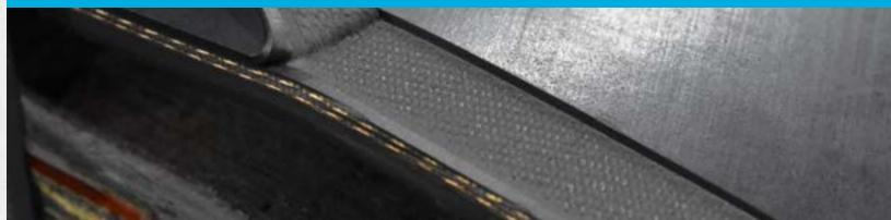
Joining the ends of conveyor belts can be achieved by a variety of methods to accommodate every application. Vulcanized splices provide a continuous, smooth and strong connection. Lacing (mechanical fasteners) are ideal for quick installations with minimum downtime. A lace pin is provided to securely connect the two ends.
